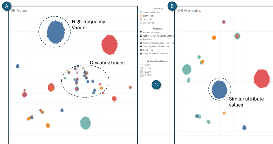
Fig. 2: Multiple coordinated view of two scatterplots showing the DR results of A) traces and B) attributes (outcome, outstanding balance, payment amount, dismissal). C) An interactive legend enables filtering. Dots in the scatterplot represent cases (i.e., traces). Jittering is used to prevent overplotting. If two dots are close, it means the traces are similar; in A) clusters of similar traces representing variants emerge (e.g., high-frequency variant) and smaller clusters of deviating traces. In B) clusters of similar attribute values emerge. Interaction enables the exploration and discovery of interactions between both representations.
